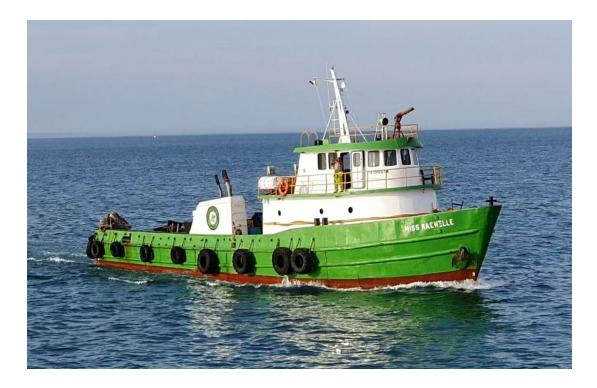
RAM / AHTS, performs bay and cabotage operations. It has a winch on deck to carry out towing operations and anchors movement, it is a very maneuverable ship, it has a useful cover area 53 mtrs2 and it has storage tanks for the transport of industrial and diesel water, all these characteristics make it a very versatile boat.
