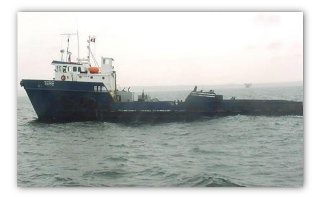
RAM / AHTS, performs bay and cabotage operations. It has a winch on deck to carry out towing operations and anchors movement, it is a very maneuverable ship, it has a useful free deck area and it has storage tanks for the transport of industrial and diesel water, all these characteristics make it a very versatile boat.
